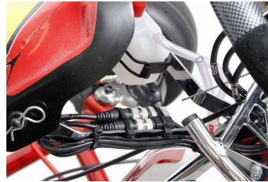
Two splitters mounted to increase number of sensors.
