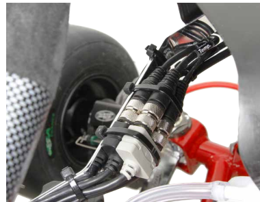
The splitters reduce the number of cables to the steering wheel.
