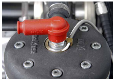
Cylinder head temperature sensor mounted below the spark plug.
