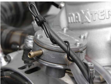
RPM wire mounted to pick up the ignition signal from the ignition wire.
