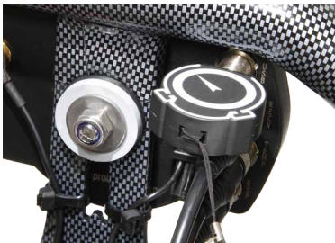
Unipro USB flash key mounted in the USB connector.
