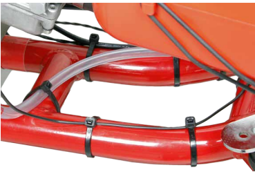
The RPM wire is running alone all the way to the ignition.
