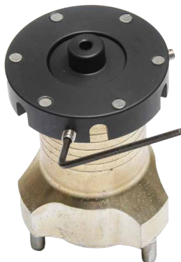
Sensor disc is fixed using the three screws and centered using the centering bush.
