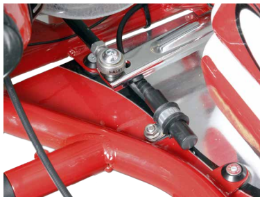
Magnet receiver mounted at the lowest point on the go-kart.
