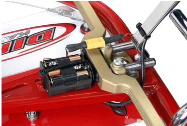
Battery holder with six AA Alkaline batteries powering UniGo. Rechargeable can be used.
