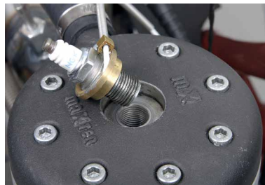
Sensor mounted instead of the washer on the spark plug.
