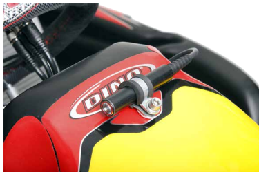
IR receiver mounter at the front, facing the right way at the finish line!
