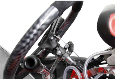
RPM wire attached with cable ties.
