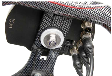
Run the RPM wire away from other cables.
