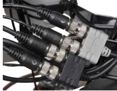
Gray splitter for temperature and black for receiver and speed.
