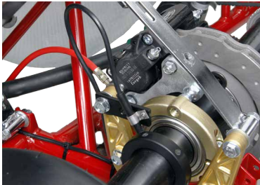
Speed kit mounted on rear axle. Notice the nice bend on the wheel sensor cable.
