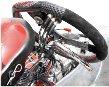
Cable fixed to the frame with cable ties.
