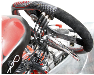
Cable fixed to the frame with cable ties.
