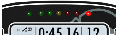
Worse LED turned on to show the laptimer is worse than the best lap time.
