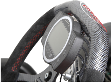
UniGo mounted at the correct distance to the steering wheel.
