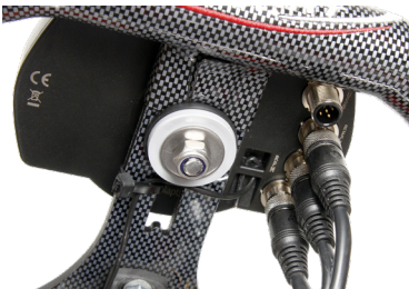
Run the RPM wire away from other cables.
