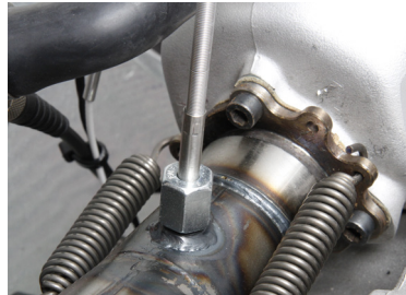
Exhaust fitting welded on the exhaust pipe.
