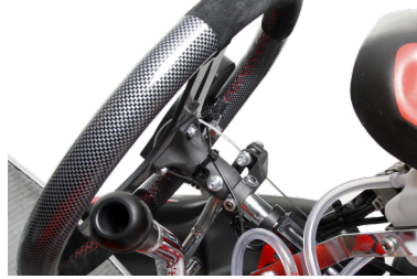
RPM wire attached with cable ties.
